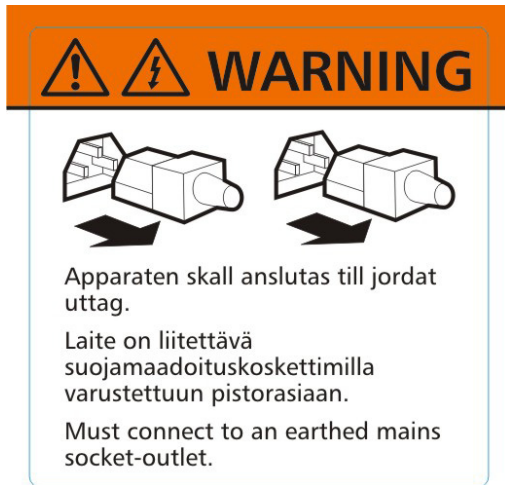
Fig. 02 - Warning Label – Earthed Mains Socket
