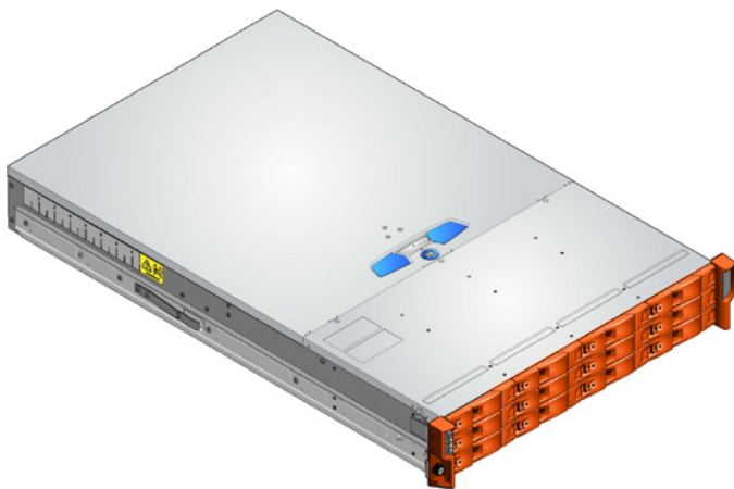
Fig. 06 - The 12big Rack Storage Server – front view
