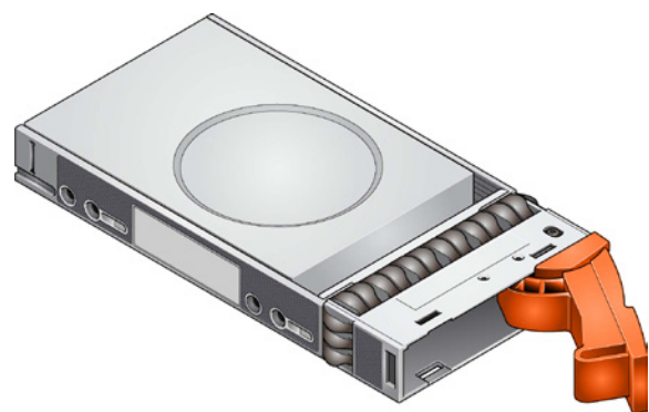
Fig. 40 - Installing a Drive Carrier Module (1)
